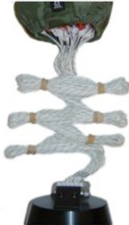
6-6 Six inch “S” folds - Retainer bands doubled
