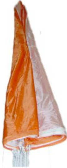
6-3 Fold canopy into thirds by folding left side half way on top of right side
