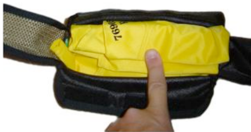
7-13 Fold remainder in half again. Should lay on top cylinder and left side bladder.
