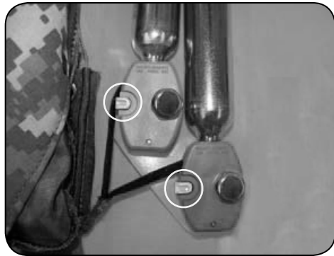
7.1.6 Installing the green safety clips.
